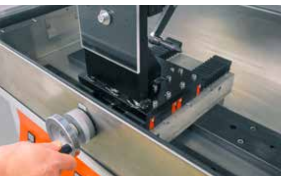
Axially adjustable working base for e.g. material quality cuts
