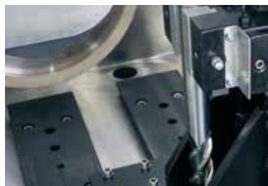
• Clamping device for slitting oil coolant holes lengthwise
