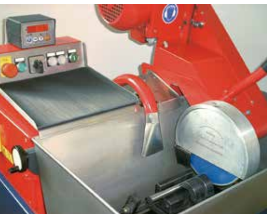
UFT 210 – the machine for cutting-off and facing
