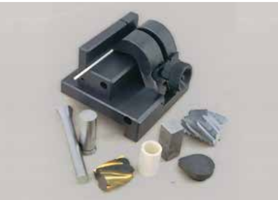
Three point clamping device for 3 – 50 mm
