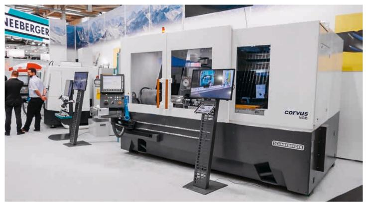
Optionally available as C or B type with 5 or 6 axes, up to 24 kW (S1) grinding performance
