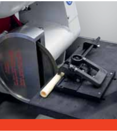
left: KT 150 detail with length stop and fast clamping device
